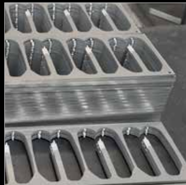
Anticorodal aluminum bars for BF1 handle production
