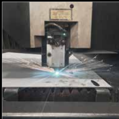
Laser cutting of a BÖHLER N690 steel sheet (thickness: 0.11 inches)
