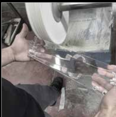
Handmade polishing of SUPPRESSOR 30° G.I.S. special box Lucidatura manuale scatola SUPPRESSOR 30° G.I.S.
