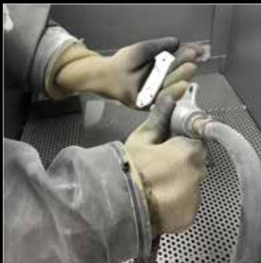
Sandblasting process of MFO handle Sabbiatura impugnatura MFO
