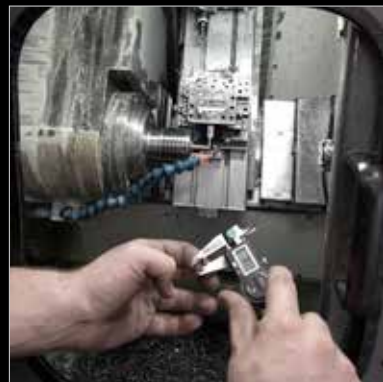
Quality control on BF line screw turning process
