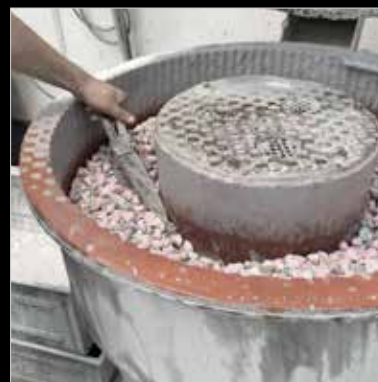
Vibration finishing of various blades
