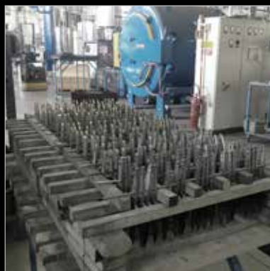
SHRAPNEL OG blades during heat-treatment
