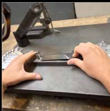
Deformation check performed on MF3 INGREDIOR blade
