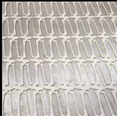
Laser-cut steel sheet showing MF3 INGREDIOR blade shapes
