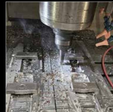
Dry milling of a Fulcrum S blade
